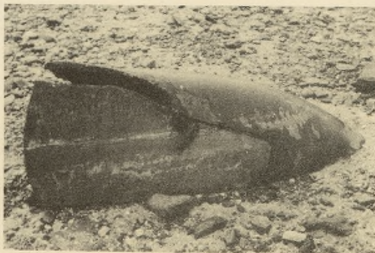
FRACTURED 12,000 lb. BOMB BODY ON FORESHORE
