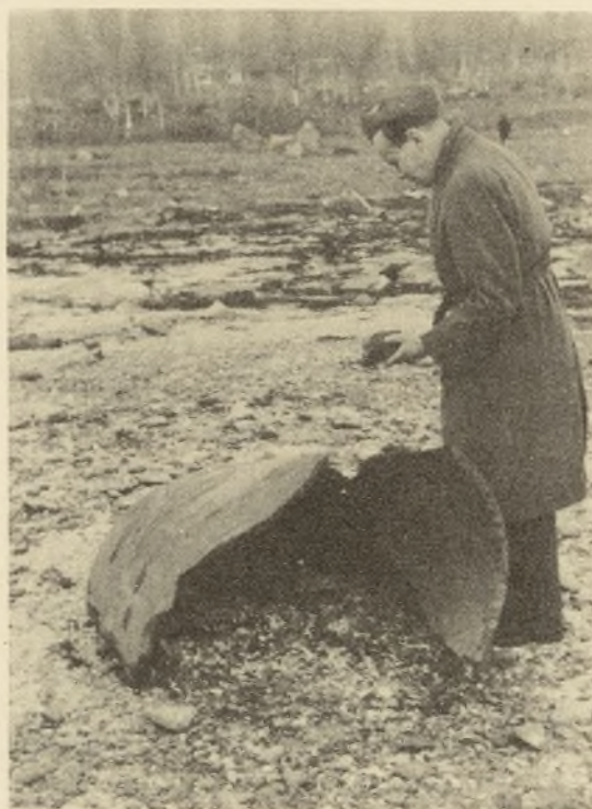
FRACTURED 12,000 lb. BOMB BODY ON FORESHORE
