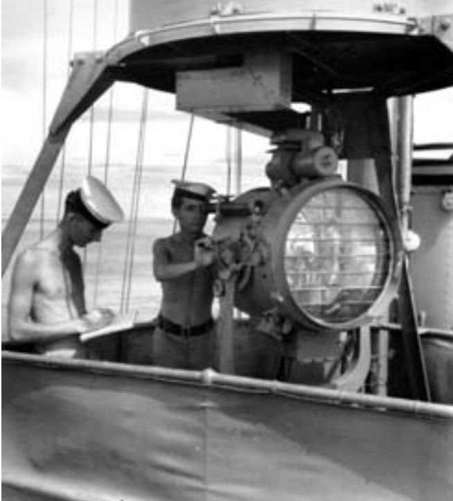
Flashing light signalling reached its peak during World War II. Here two RAN ratings operate a 20-inch pattern 170 A signalling projector
