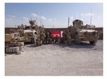
Figure 4 – Armoured Vehicles, the one on the left having a Mine Roller to sweep for IED.
