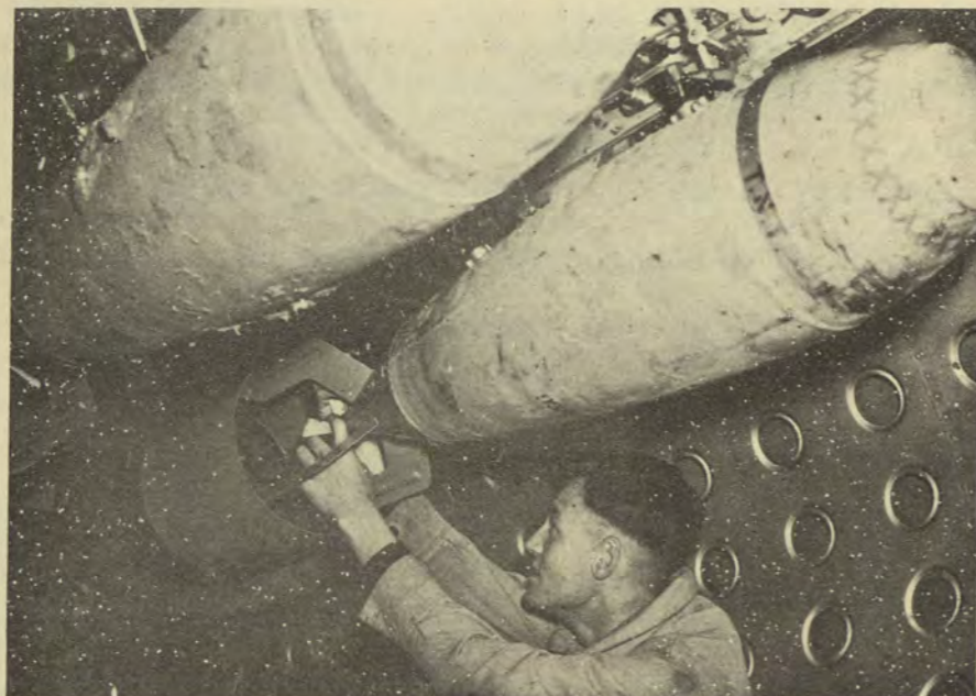
After bombing up, the armourer checks the fusing links and tail pistol of the bomber. These are 500-pounders.
