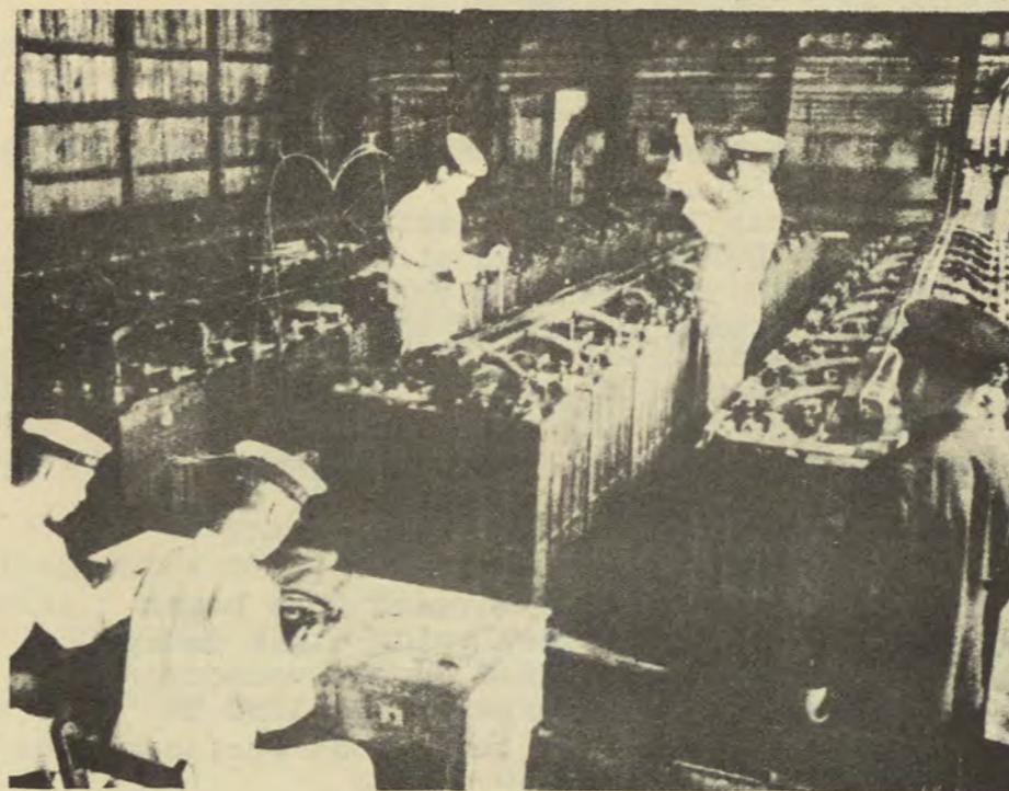
Batteries — the source of motive power when the submarine submerges. Japanese ratings learn how to maintain giant storage batteries prior to passing out.
