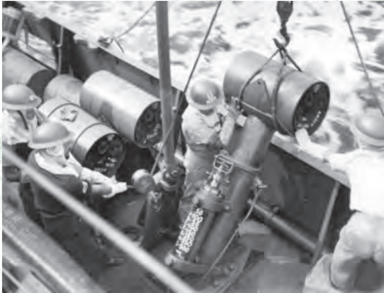
The crew of HMAS Castlemaine manually reload a depth charge thrower. Time was of the essence between depth charge attacks and the speed at which a weapon could be reloaded could often make the difference between destroying a contact and it getting away.
