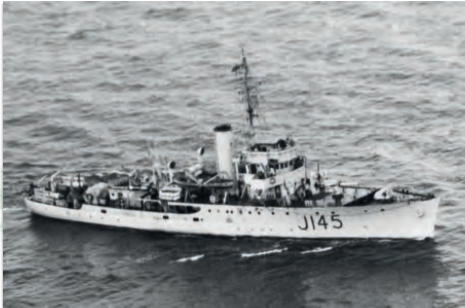
HMAS Lismore's bridge superstructure differed from other vessels of the class with the addition of a 'monkey island' above the bridge. During World War II she saw extensive service in the Indo-Pacific, Mediterranean Sea and in waters off Okinawa in 1945. She was awarded the following campaign awards: INDIAN OCEAN 1941-44, SICILY 1943, PACIFIC 1945 & OKINAWA 1945.
