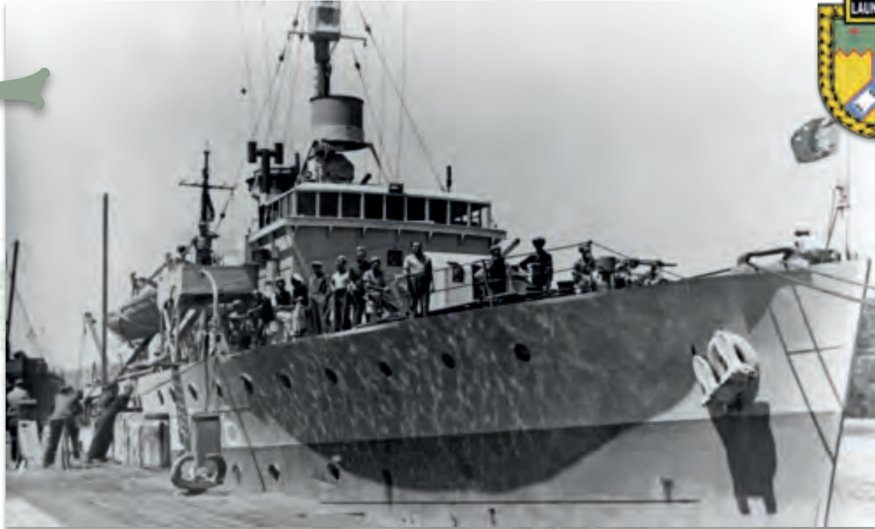
HMAS Launceston was the first RAN ship to carry the name of the northern Tasmanian riverside city. Here she can be seen in her late war paint scheme and equipped with her radar 'lantern' atop the bridge. Launceston commissioned at Brisbane on 9 April 1942.
