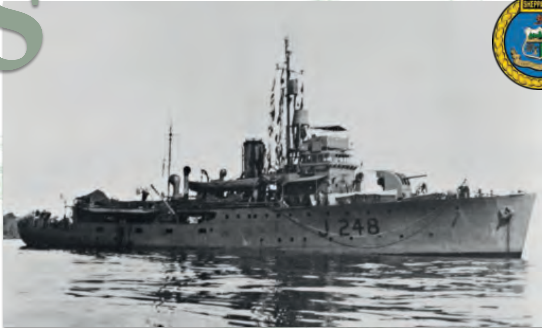
HMAS Shepparton was another of the Bathurst class corvettes modified to include a 'monkey island' atop the bridge. This may have been in connection with the survey duties she undertook prior to the US landings at Humboldt Bay, Tanamarah Bay and Aitape in New Guinea in 1944.
