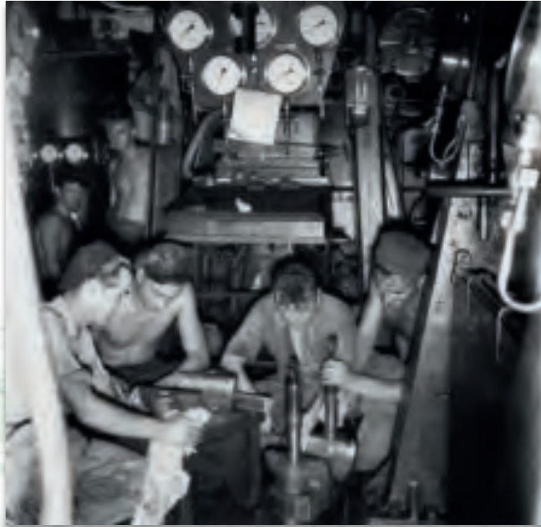
Above: Engine room personnel working hard to rectify a defect on a main engine bearing.
