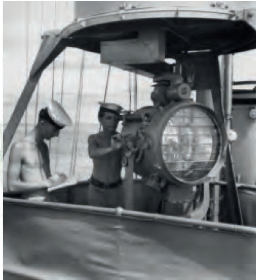
Left: Signalmen Harry Edenborough and Graham Collier of HMAS Rockhampton closed up on the 20 inch signalling projector atop Rockhampton's bridge. Above: HMAS Broome's 4-inch gun crew undertaking loading drills on her foc'sle.
