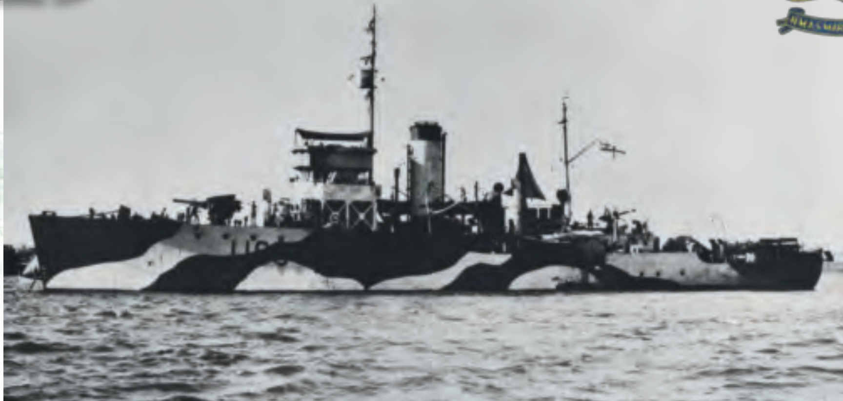
HMAS Maryborough was built by the Walkers Yard at Maryborough in Queensland, the town after which she was named. Here she can be seen wearing her early war camouflage paint scheme that very effectively breaks up the silhouette of the ship. Note the distinctive bridge superstructure that differed from many of her sister corvettes.
