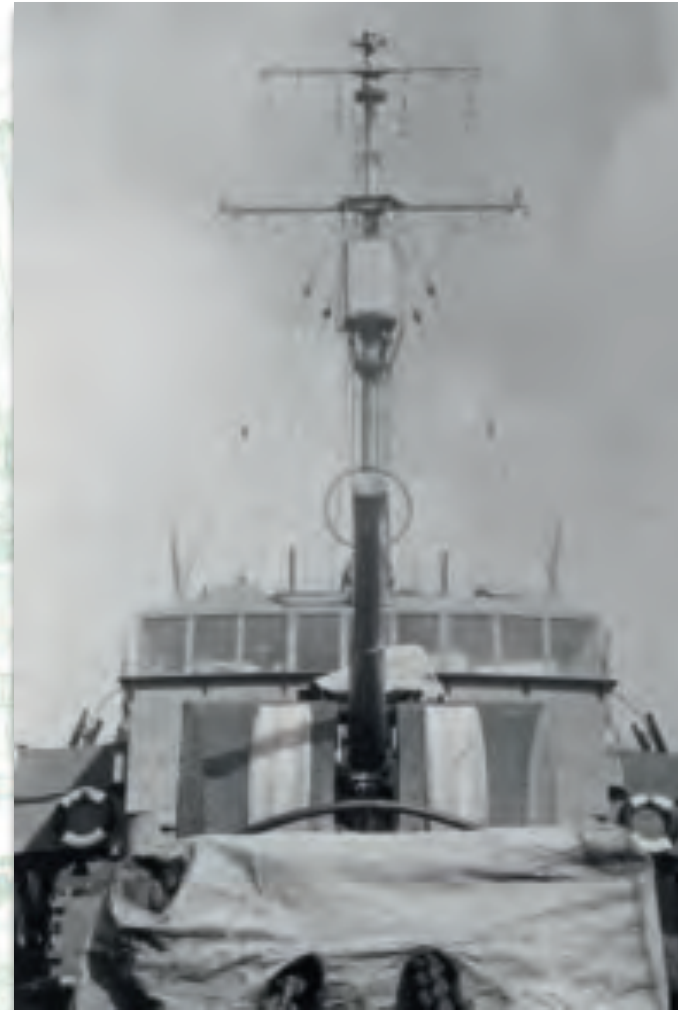
Left: Working aloft to maintain rigging and wires, supporting the mast and yardarms was a routine part of shipboard life. Right: Looking aft from the foc'sle of an early war Bathurst class corvette. The configuration of the mast and yardarms is clearly visible in this pre-radar equipped ship.
