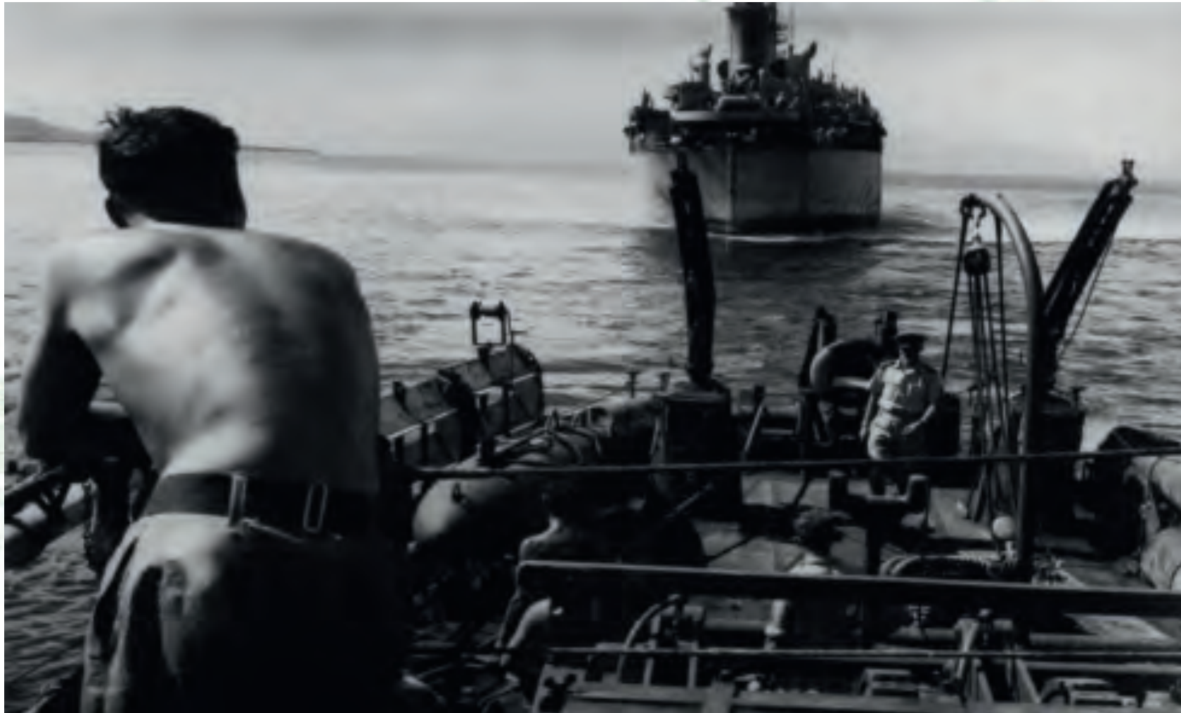
An officer and ratings monitoring a towing hawser rigged on the quarterdeck of HMAS Broome. Although powered only by a triple expansion steam engine, the Bathurst class corvettes were capable of attaining a top speed of 15 knots.
