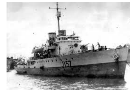
HMAS Toowoomba . Note the Type 271 radar "lantern" above the bridge, no S/L and what appears to be a 12-pdr on the foredeck. [ navy.gov.au ]
