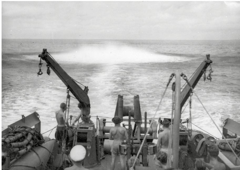
Depth charge or charges exploding in the wake of a Bathurst Class corvette. [AWM P00782.003]
