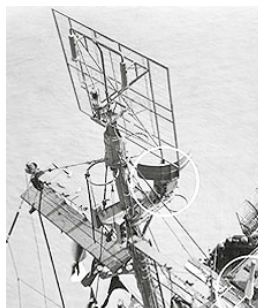
US Type SC-1 (air-warning) top and SG (surface warning) antennas circled. [Pacific War Online, National Archives 19-N-40832]
