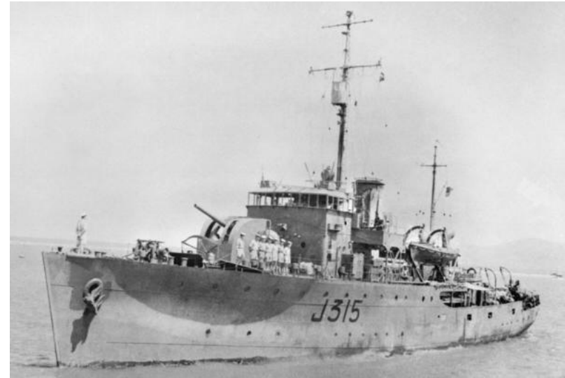
HMAS Wagga . Note no radar apparent but the 4-inch Mk XVI is fitted. [AWM 041254]
