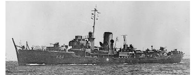
HMS Hyacinth without extended forecastle with 12-pdr 12 cwt QF or QF 4-inch Mk XIX and Type 271 radar. [commons.wikimedia.com]
