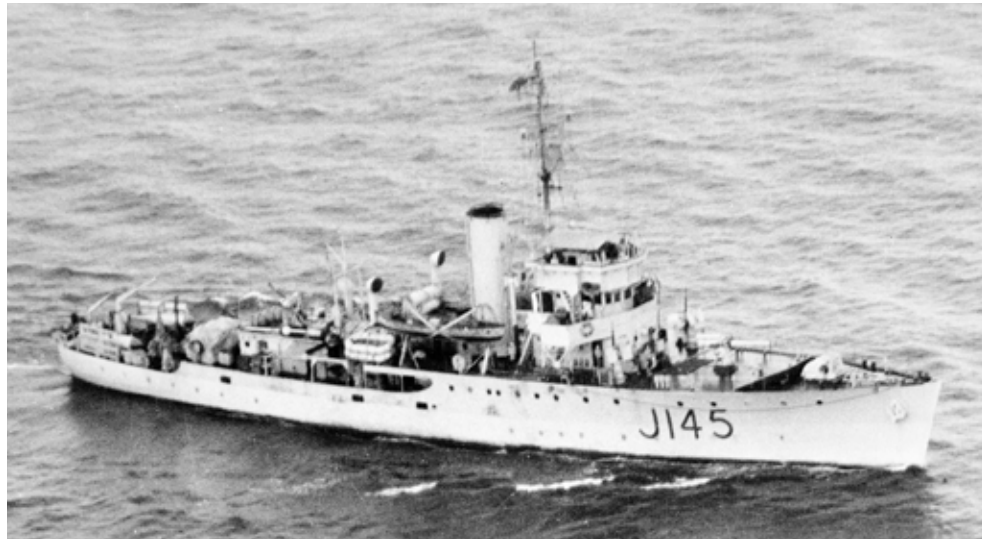
One of the few photos of HMAS Lismore . The 4-inch BL Mk IX is without a shield but 20mm Oerlikons are present on the foredeck, forward of the bridge structure. [navy.gov.au]
