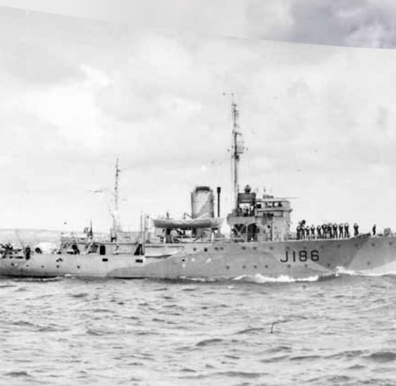
HMAS Ipswich . Note SW1C type radar antenna at masthead. [AWM P00433.007]
