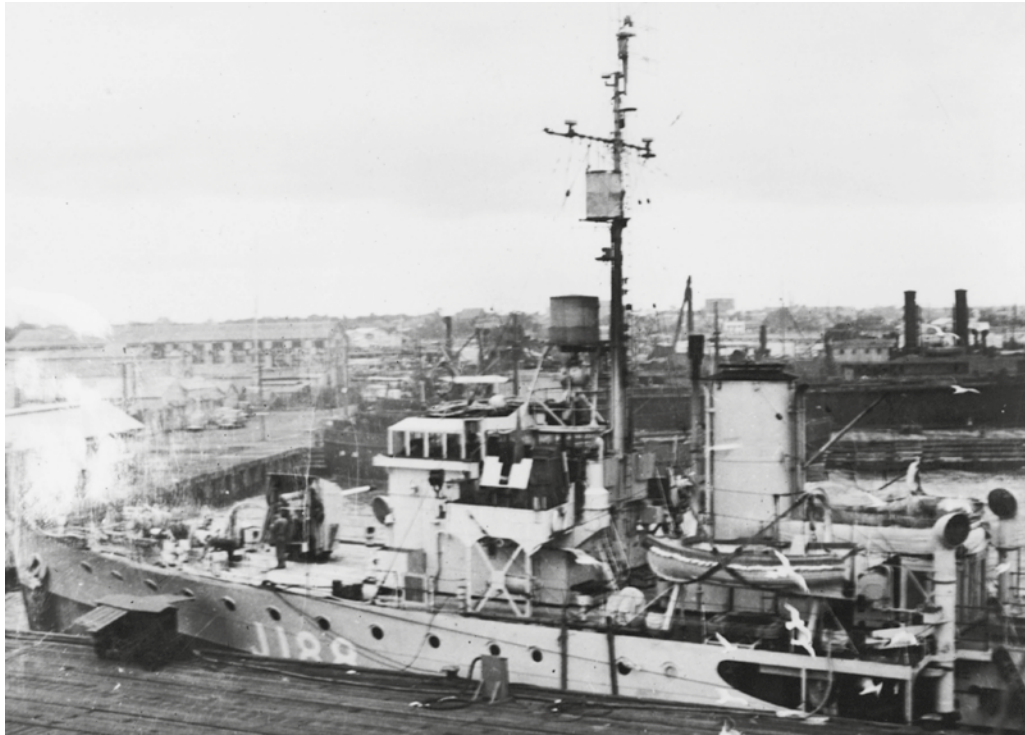
HMAS Gawler . Note the A286 antenna is mounted aft of the mainmast. Note the ladders giving access to the signal deck and bridge. [navy.gov.au]
