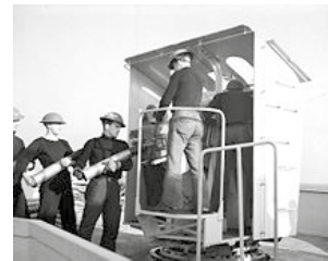
QF 4-inch Mk XIX on a CP Mk XXIII mounting. [Library & Archives Canada LAC 3206297]
