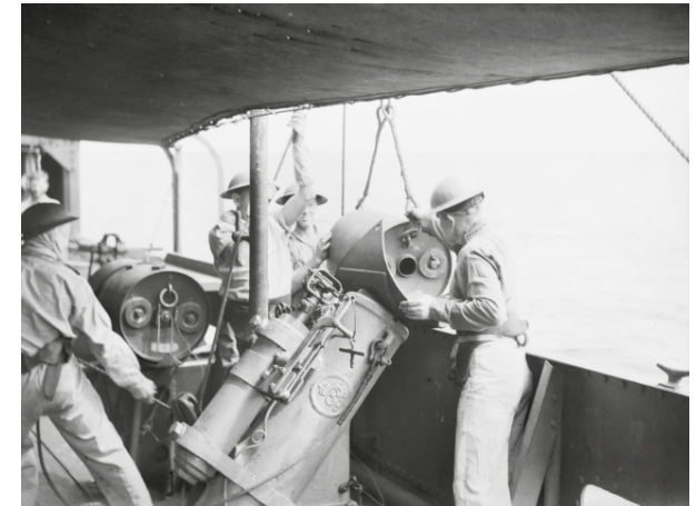
Thornycroft type Mk II depth charge thrower being loaded on a corvette. Quite a lot of teamwork was required to lift these charges and position them, especially in a seaway. [AWM 075719]
