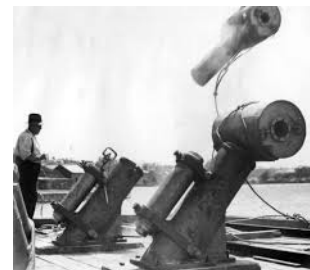
Dummy depth charge test firing in Sydney. Note the arbor starting to separate from the depth charge. [AWM H98.105/3034]
