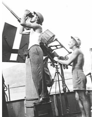
20mm Oerlikon on a pedestal mounting on the bridge wing of a corvette. How did this high trunnion work for surface targets? [AWM O26614]
