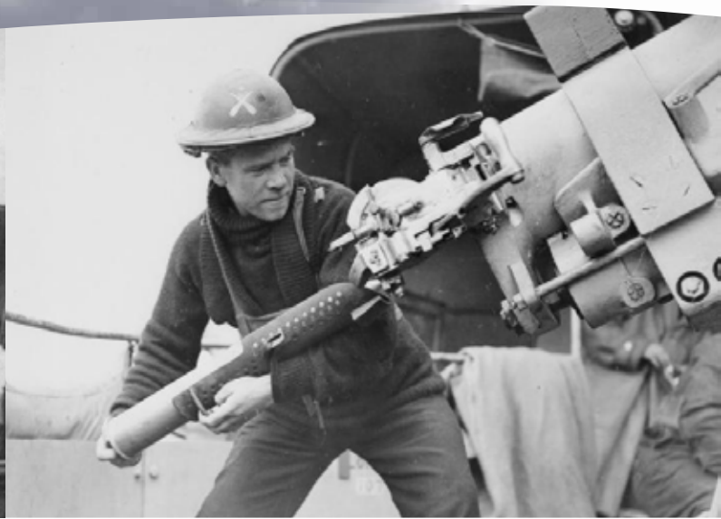
12-pdr 12 cwt QF being loaded. Note the holder with separate charge and projectile. [commons.wikimedia.com]
