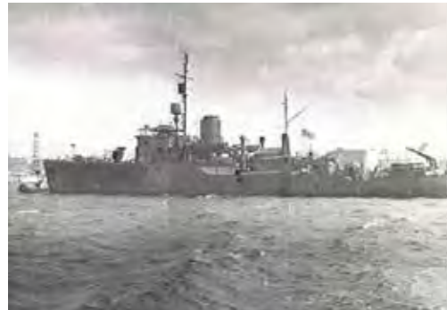
HMAS Broome . Note 12-pdr still fitted yet she now has the full radar fit-out. [AWM 300469]
