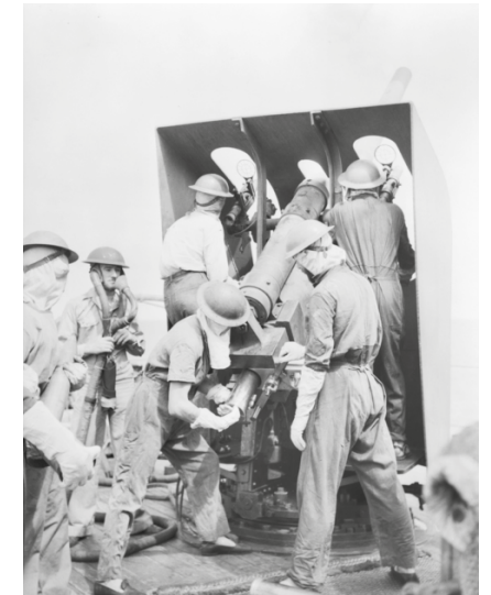
The gun crew of a QF 4-inch Mk XIX with the gun at maximum elevation. [AWM 075718]
