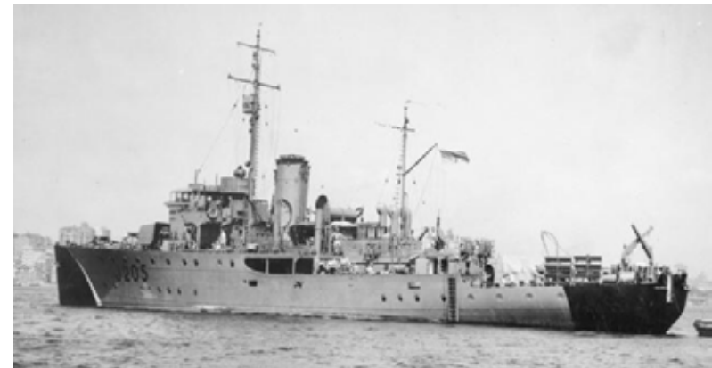
HMAS Townsville . Note camouflage to “blackout” the bow and stern and give a false impression of the ship’s length. [ navy.gov.au ]
