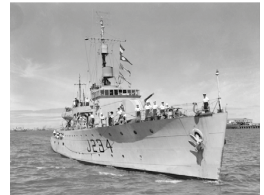
HMAS Latrobe . Note the single QF 4-inch Mk XVI on a Mk XX mounting; a peculiarly Australian weapon. [AWM 300954]
