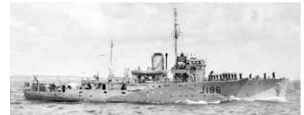
HMAS Ipswich . Note SW1C type radar antenna at masthead. [AWM P00433.007]
