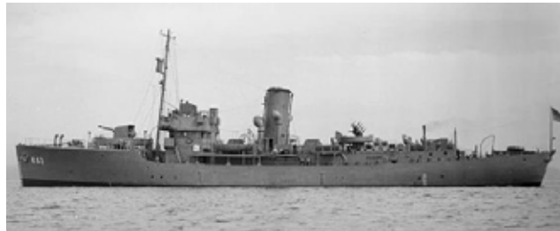
HMS Picotee . Note the unusual fitting of a quad .5” MG in place of the usual 2-pdr. [commons.wikimedia.com]
