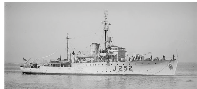
A later photo of HMAS Echuca with full radar and 20mm Oerlikon secondary armament fit-out. [State Library of Victoria Allan Green Collection]
