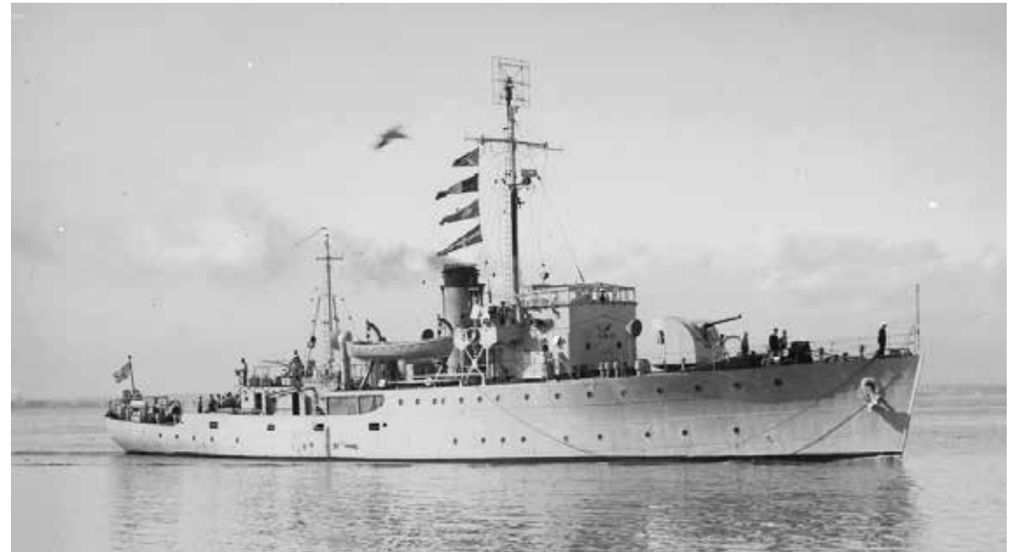
HMAS Gladstone without pennant number, QF 4-inch Mk XVI and no minesweeping gear apparent. [State Library of Victoria Allan Green Collection]
