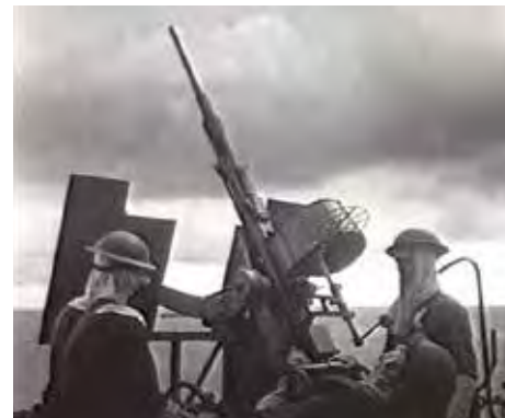
An Oerlikon crew HMAS Rockhampton . Note the crew are wearing anti-flash gear. The seaman on the left adjusts the trunnion height via a wheel. The one on the right changes the 60-round magazines. [AWM 108649]
