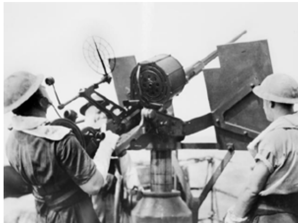
20mm Oerlikon on a Mk1 (US Mk 4) mounting. Note that the wheel on the left-hand side raises the whole gun. [AWM P00444.061]
