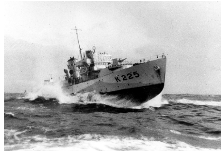
The Flower Class corvette HMCS Kitchener somewhere in the Atlantic. Note the cut away forefoot from her whaler heritage. [wikivisually.com]
