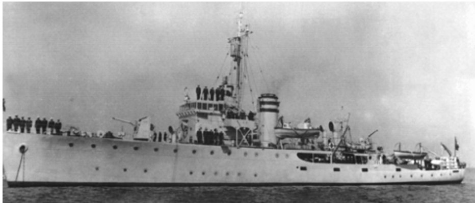
HMAS Launceston , probably post War. Note no apparent 20mm in bridge wings, mainmast reduced to a frame, no pennant number and flotilla bands on the funnel. [navy.gov.au]
