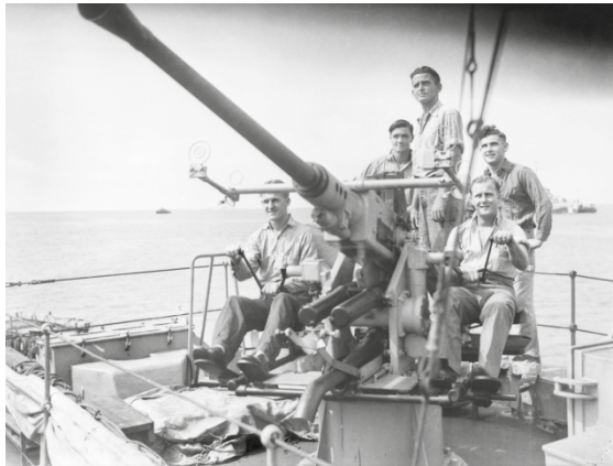
40mm Bofors Mk III on a raised mounting on a corvette. [AWM 109987]
