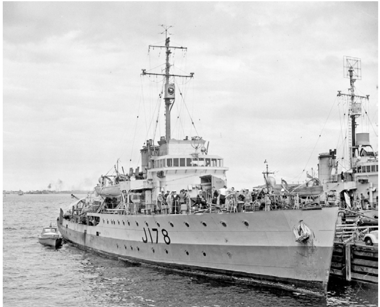
HMAS Geraldton with Type 291 radar at masthead, no S/L and flying Bridge. [navy.gov.au] [AWM 045137]
