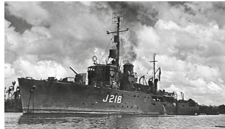
A 1944 photo of HMAS Kapunda showing the QF 4-inch Mk XIX on the Mk XXIII mounting and full radar fit out but retaining the dark blue-grey overall camouflage – probably similar to the USN's. [AWM 300857]
