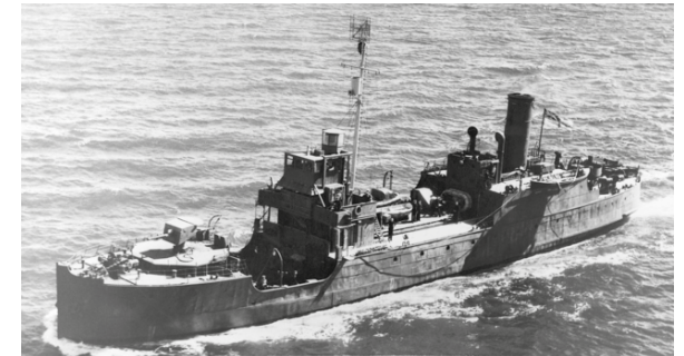
HMAS Kybra showing American SC or Australian A286Q antenna at masthead and a Type 271 above the bridge. To further confuse the nomenclature issue, when conducting radar trials in early 1943, official Kybra records describe these as A79 and A272 respectively! [AWM 300939]
