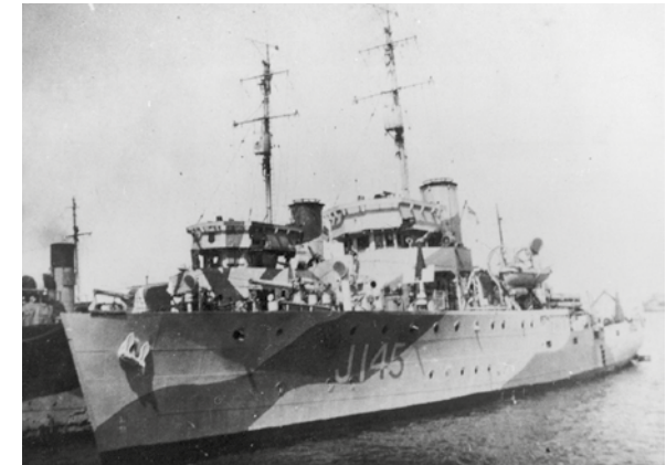
HMA Ships Lismore and Maryborough in Tunis, 1943. Note what appears to be SW1C type radar antenna at the masthead and pedestal-mounted 20mm Oerlikon forward of their taller bridges. [source unidentified]
