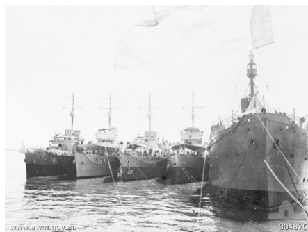
HMA Ships Toowoomba , Lismore , Burnie and Maryborough beside a depot ship, most probably HMS Lucia , at Ceylon in mid-November, 1944 before departing the British Eastern Fleet for Australia. Note that Toowoomba and Burnie both have the distinctive Type 271 "lantern" above the bridge and Lismore and Maryborough may have the Type 291 at the masthead. [AWM 304875]
