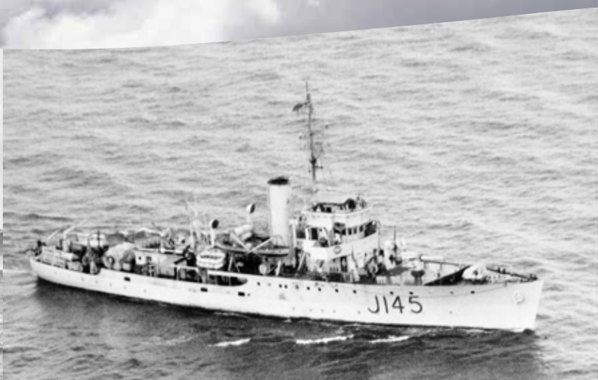
One of the few photos of HMAS Lismore . The 4-inch BL Mk IX is without a shield but 20mm Oerlikons are present on the foredeck, forward of the bridge structure. [navy.gov.au]
