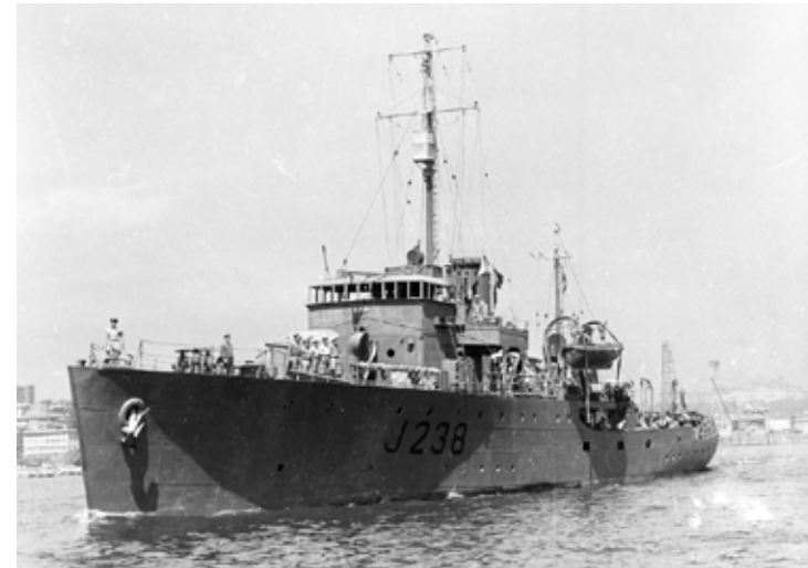
HMAS Gympie . Note there is no radar fitted and the 12-pounder has an extended shield. [navy.gov.au].
