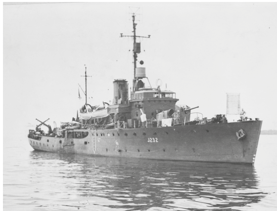
HMAS Deloraine . Note the non-standard sized pennant number, no apparent guardrails forward of the breakwater, scrambling net deployed and black ball in rigging indicating at anchor. [AWM 041255]
