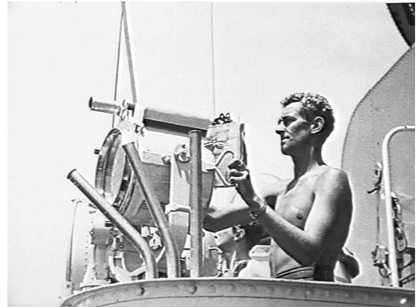
A 10-inch signalling lamp in use. Note the telescope and the signals pad. [AWM 304775]
