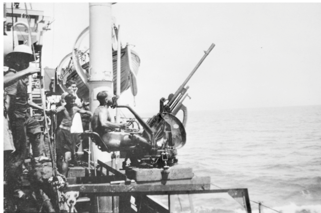
Captured Italian Breda Model 35, 20mm cannon on HMAS Lismore . Where did the loader stand? [AWM P0431.001]
