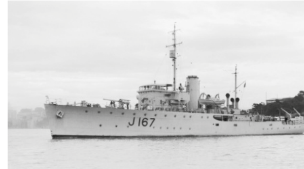
HMAS Goulburn in Sydney in an AWM photograph on 28 Feb 1941 on the day of her commissioning. Note that the 20-inch searchlight may be of the type shown in the 137/4/4 drawing or duplicated in each bridge wing. Note that the bridge wings appear smaller and taller than what would be regarded as standard in both photographs. Photographs of Burnie indicate that she was similar. [AWM 300709]
