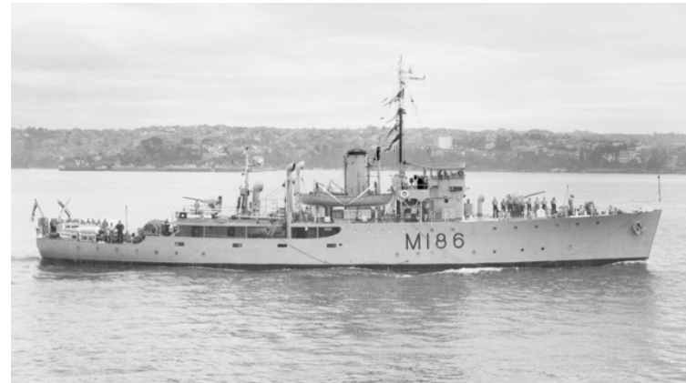
HMAS Cootamundra with 40mm Bofors fore and aft, US SG radar on shorter foremast. Probably post recommissioning 12 December 1951 as training ship. [AWM 300554]
