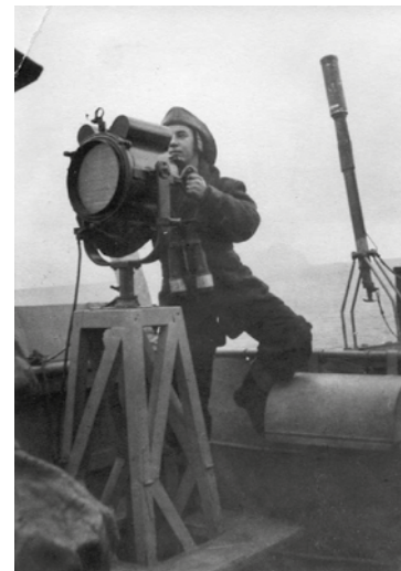
PAC projector on a Canadian corvette. (source unidentified or unestablished)
