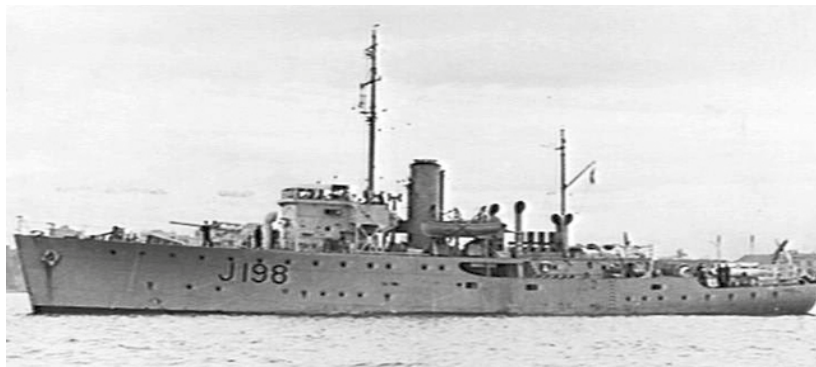
HMAS Burnie as completed. Note: Small bridge wings, no apparent searchlight/s, no secondary armament. [AWM 3921887]
