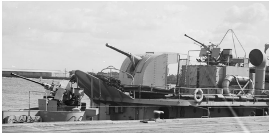
4" Mk XVI on single Mk XX mount on a RAN frigate. [State Library of Victoria SLV H91.250]
