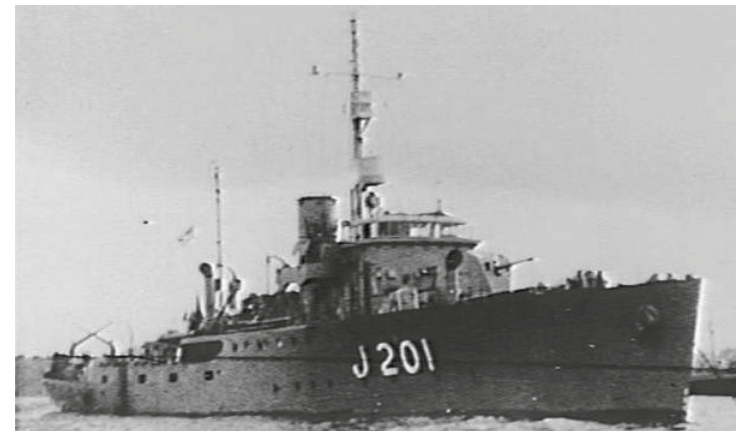
HMAS Geelong with later modifications including QF 4-inch Mk XIX on Mk XXIII mounting and full radar fit out. AWM photograph recorded as Broken Bay, 1942 but it is most unlikely that this radar fit would have been available at this time. [AWM P01311.001]
