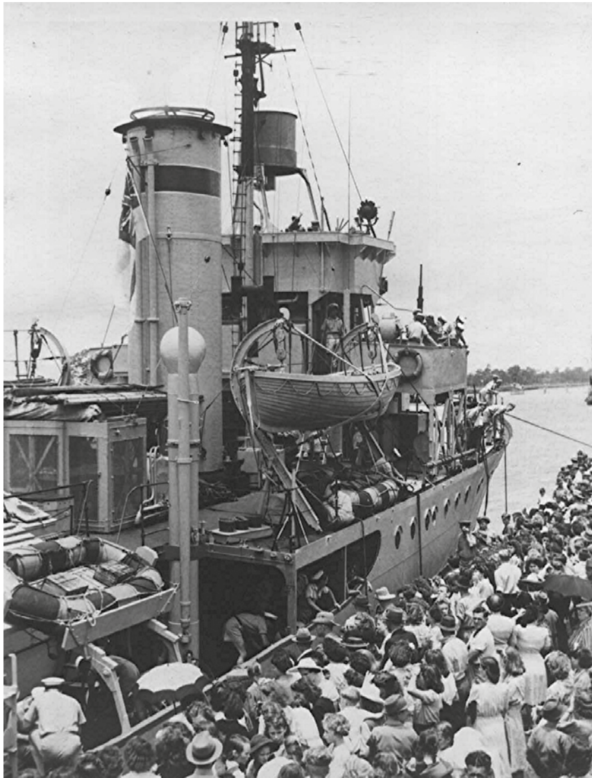
HMAS Maryborough visiting her namesake city, Dec 6 1945. Note the taller funnel to clear the taller bridge. [Shipbuilding At Walkers Limited]
