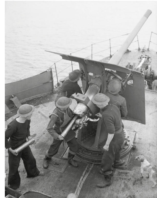
12-pdr 12 cwt QF. Note the second loader has a charge only. [commons.wikimedia.com]
