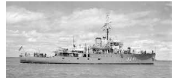
HMAS Bunbury in late-War or post-War configuration with open bridge and US SG radar on foremast. [AWM 125071]
