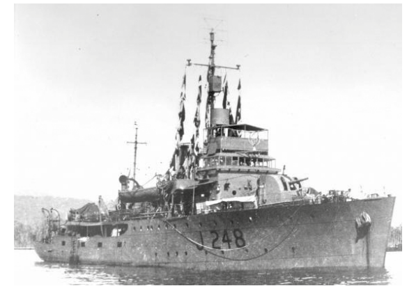
HMAS Shepparton as a survey ship with flying bridge. Note davits for extra ship's boat, aft. [navy.gov.au]
