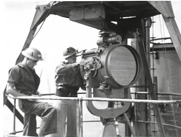
20" searchlight/signal projector, HMAS Geelong . The A272 radar antenna is mounted above the searchlight platform. [AWM 075724]
