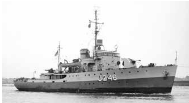
HMAS Fremantle without any minesweeping gear as anti-submarine escort. Note the single-barrelled version of the QF 4-inch Mk XVI on the foredeck. [navy.gov.au]
