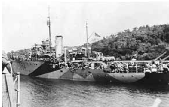
HMAS Ballarat . Note no radar apparent and what appears to be a 2-pdr aft of the mainmast. [AWM 106652]
