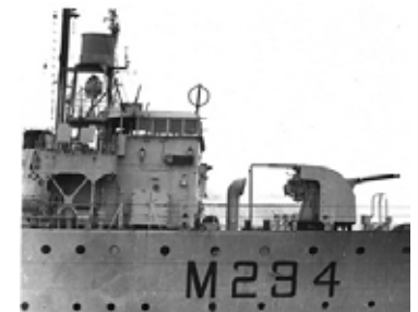
HMAS Latrobe bridge showing A 272 radar with what might be a Type 242 IFF interrogator in front. Note the 20-inch searchlight, PAC projectors, RDF loops, RU locker beside bridge. Catch net for 4" Mk XVI on MkXX mounting with depression rail forward. [Eric Hogben Collection 5701]
