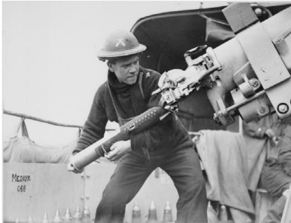
12-pdr 12 cwt QF being loaded. Note the holder with separate charge and projectile. [commons.wikimedia.com]
