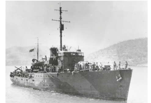
HMAS Armidale . Note what appears to be Canadian type SW1C radar at masthead. [AWM 026612]
