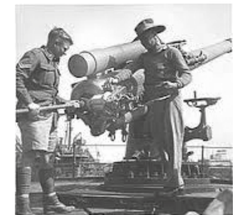
4-inch/45 BL Mk IX on a CP Mk I mounting. No shield. [AWM 023669]
