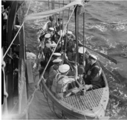
Boarding party being lowered in 27 Montagu whaler. Note the tiller is operated by a yoke ahead of the step for the mizzen mast. [wikivisually.com]
