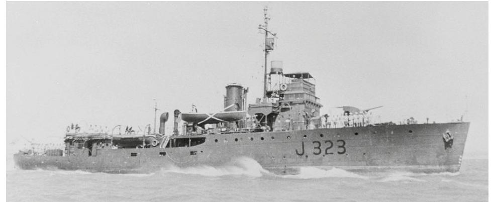
A later photo of HMAS Benalla showing what might be two 20mm Oerlikons on the centreline of the extended deckhouse, prior to the fitting of the 40mm Bofors shown in the drawing. Note the flying bridge. [navy.gov.au]
