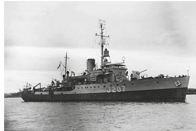
A 1945 photograph of HMAS Mildura at Tarakan with a QF 4-inch Mk XIX on a Mk XXIII mounting forward, a 40mm Bofors aft, full radar fit-out, RDF loop ahead of the bridge and a two-tone BPF type camouflage scheme. [AWM 110292]
