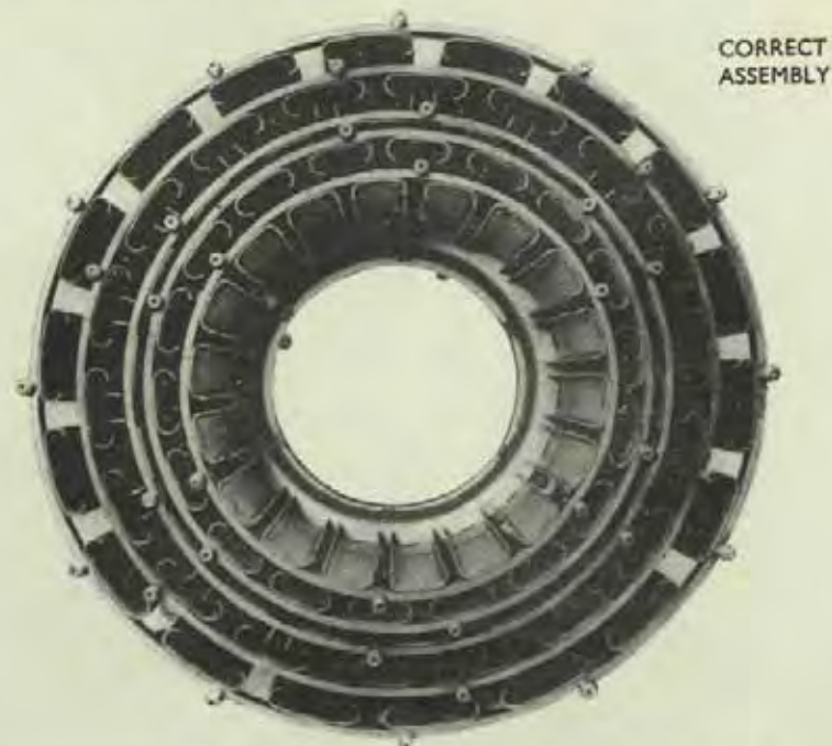
Fig 2. Correct Assembly showing outer two rings of vanes in staggered radial alignment.
