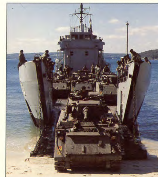
ABOVE: An Army fire support vehicle drives off an LCH's bow ramp onto a beachhead. LEFT: HMAS BETANO, one of the RAN's six heavy landing craft.
