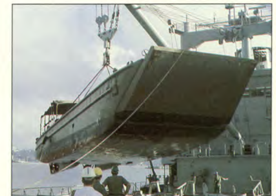
ABOVE: An Army LCM 8 landing craft is lifted from HMAS TOBRUK by the ship's own heavy lift derrick.
