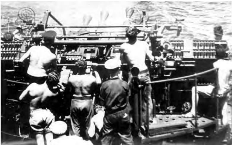
A 2-pdr Mk VIII pom-pom in action. These weapons were hand elevated and trained, and the controlled rate of fire was 96-98 rounds per minute.
