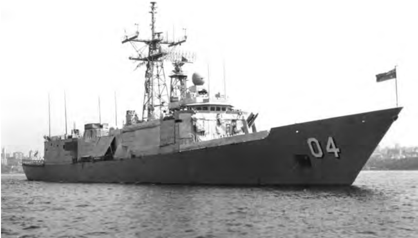
HMAS Darwin with RAM panels, March 1991 (J Mortimer)
