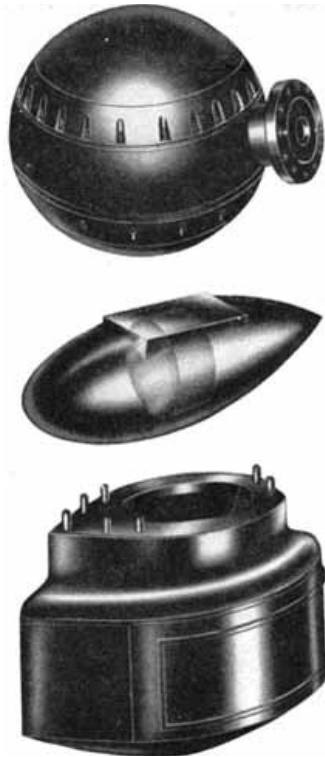
Figure 1: Standard WWII sonar domes (Bureau of Naval Personnel, 1953)
