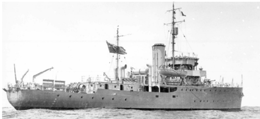
The lead ship, HMAS Bathurst, on trials, but already fitted for minesweeping
