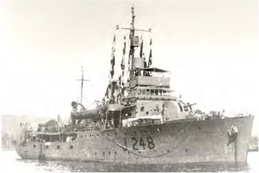
HMAS Shepparton fitted out as a survey vessel, with radar, an extra bridge and bamboo survey markers
