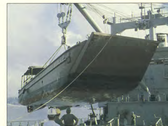
ABOVE: An Army LC 8 landing craft is lifted from HMAS Tobruk by the ship's own heavy lift derrick.
