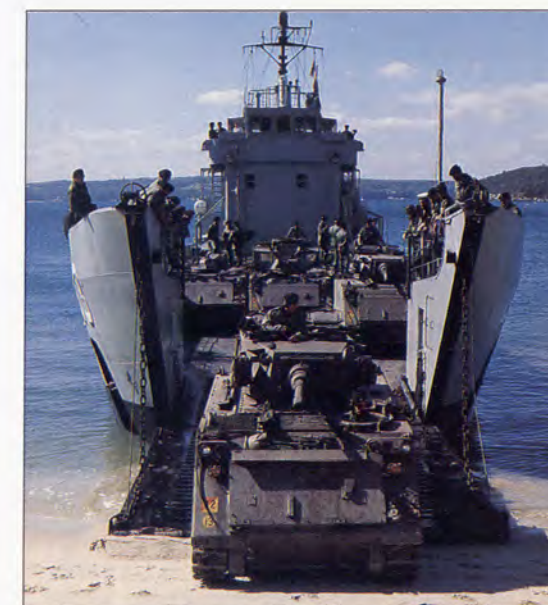
ABOVE: An Army fire support vehicle drives off an LCH's bow ramp onto a beachhead.
