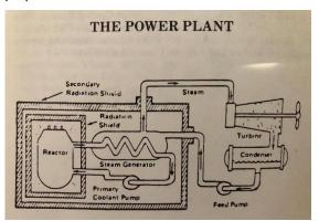
A basic diagram of the two separate closed systems that interact to propel a submarine through the water.
