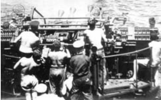
A 2-pdr Mk VIII pom-pom in action. These weapons were hand elevated and trained, and the controlled rate of fire was 96-98 rounds per minute
