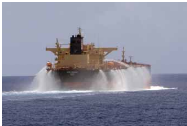
The 115,500 dead weight tonne tanker MV Dubai Princess spraying water in an attempt to prevent pirates boarding (RAN)
