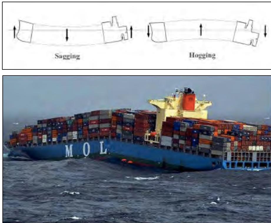
Figure 6: Sagging and Hogging of Ship Hull and Hull Failure (Source: Constanta Maritime University)
