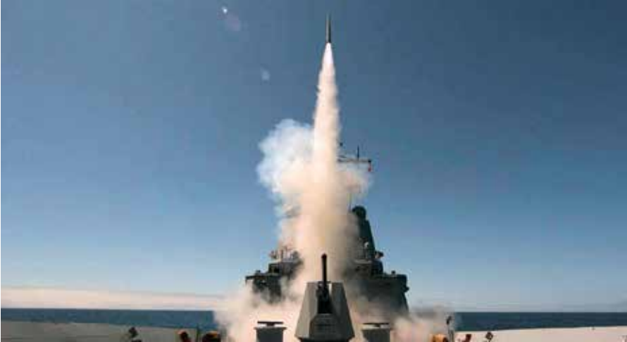
HMAS Sydney fires an Evolved Sea Sparrow Missile for the first time during Combat System Sea Qualification Trials in the Southern Californian Exercise Area off the coast of the United States.
