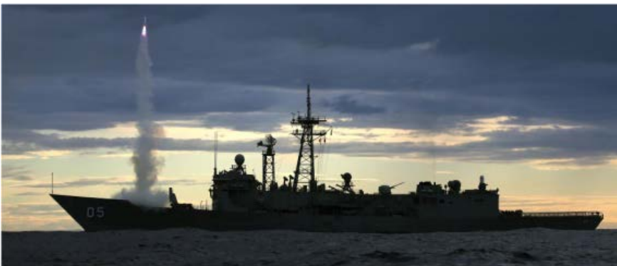
An Evolved Sea Sparrow Missile fires from HMAS Melbourne's MK-41 vertical launcher during training in the East Australian Exercise Area off the New South Wales coast.
