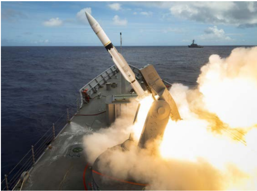
HMAS Melbourne fires a Standard Missile 2 from its Guided Missile Launching System during RIMPAC 2018.
