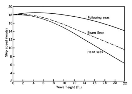
Figure 5: Performance curves for head, beam and following seas
